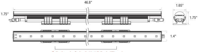
Optimal spacing for bracket installation is 16" apart.
