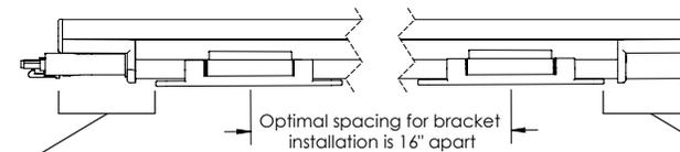
**TO PREVENT VOIDING THE WARRANTY, DO NOT INSTALL BRACKETS WITHIN 2" OF THE ENDS OF FIXTURE.**
