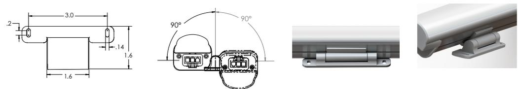
**IMPORTANT FOR 4' FIXTURE:** Affix brackets, one on each side of fixture, between center and 22".
