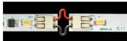
**NOTE:** POSITIVE Symbol (+) always has to be aligned on the same side for each connected LED Strip.
