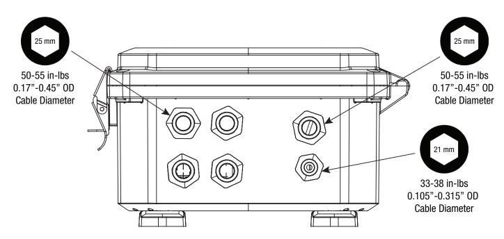
**NOTE**: Failure to properly torque watertight strain-reliefs can result in water ingress. Do not install in locations prone to flooding. For ease of maintenance, mount in locations easily accessible
