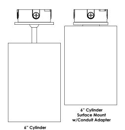
Surface Mount Conduit Adapter can be added to any of the AC, CM, SF and SPM Mounts
